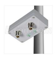
The HyperAmp® HA2401G series improves range by delivering full transmit power directly at the antenna where it is most effective. In addition the unit's receive gain compensates for cable losses. The unit can be configured to deliver the full transmit power with as little as 1 mW of input power, permitting cable runs of several hundred feet with no degradation in operating range.
