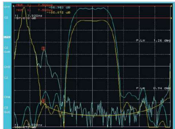
Comparison of GATE ON and GATE OFF at Frequency Axis and Time Axis
