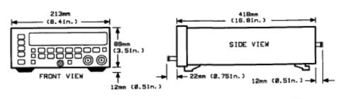
Note: For ordering cabinet accessories, the module sizes are 3-1/2H, 1/2MW, and 17D.
