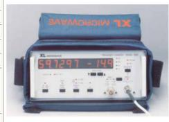
**Note:** Counter models below 40 GHz have a single Band 1 frequency range of 10 Hz to 120 MHz. Counter models at 40 GHz and above have a dual Band 1 frequency range.
