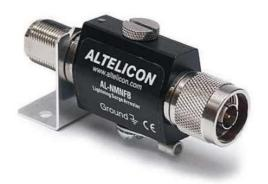
Due to its low cost and superior RF performance, this unit is ideal for IEEE 802.11b and 802.11g Wireless LAN applications, as well as ISM, MMDS, Cellular, and PCS applications. Since this protector will pass DC, it is suitable for applications where DC is carried through the coax cable, such as remote amplifiers and LNAs.
